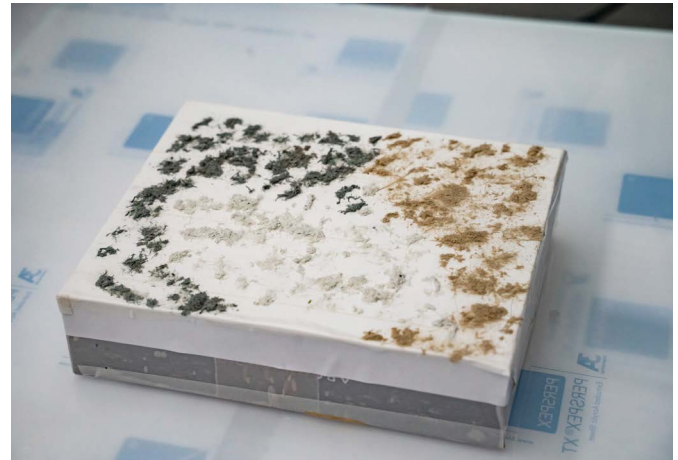
Shredded sheet of material (free asbestos fibres) on double adhesive tape
