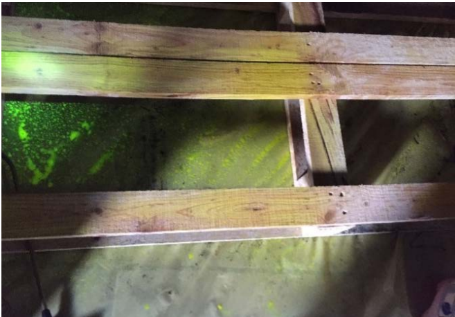
Fluorescence by illumination with UV lamp on tree and plastic in roof
