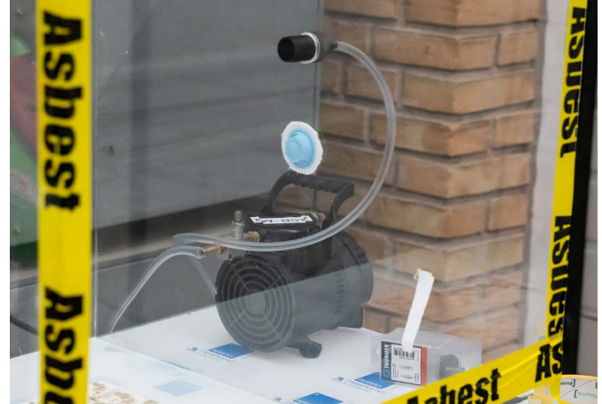
Measuring equipment connected to box for measuring airborne asbestos
